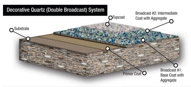
Decorative Quartz Double Broadcast System is a decorative, multi-lift, high strength concrete resurfacing system. It is used for environments requiring an attractive, high performance floor or when a concrete floor has sustained damage requiring a textured 1/8" surface restoration.
